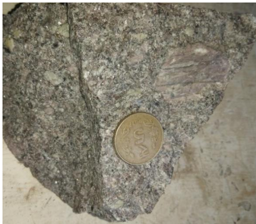
Figure. 15: Porphyritic medium grained grey granite consisting of phenocryst of feldspar of greater than coin size.
