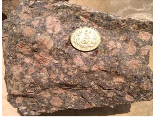
Figure. 12: Coarse grained granite showing rounded grains of feldspar.
