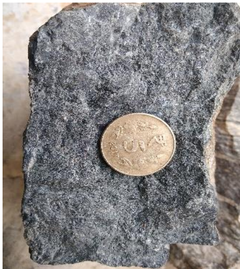
Figure. 7: Amphibolite rocks consisting of grains of tremotite and actinolite.
