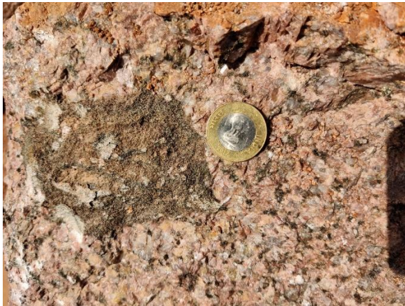
Figure. 13: Porphyritic coarse grained pink granite with large phenocryst of k-feldspar.
