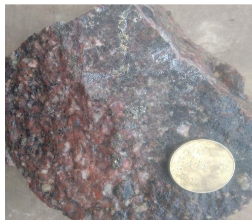
Figure. 16: Porphyritic medium grained pink granite showing stains of chalcopyrite near prithvipur area.
