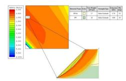
Figure 14: Calculated factor of safety of slope by Morgenstern-price method.
