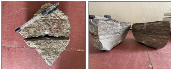
Photograph 2 Sample after PLT perpendicular to anisotropy
