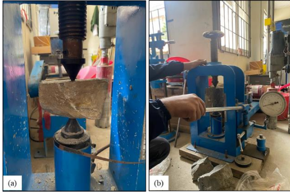
Photograph 1 (a) Close view of Point Load Machine, and (b) Full View of Point Load Machine.
