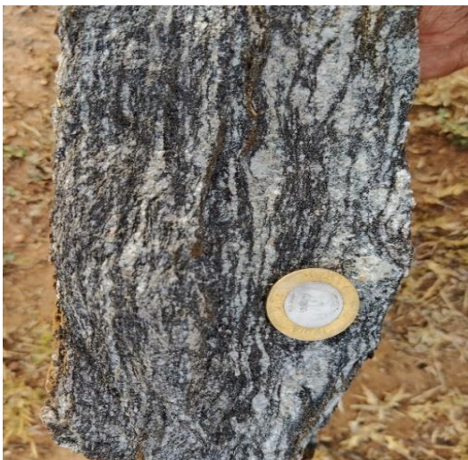
Figure 3: Biotite gneiss showing alternate banding of light and dark coloured minerals forming S-C planes.
