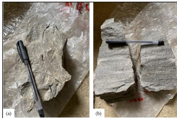
Photograph 3 Sample after PLT parallel to anisotropy
